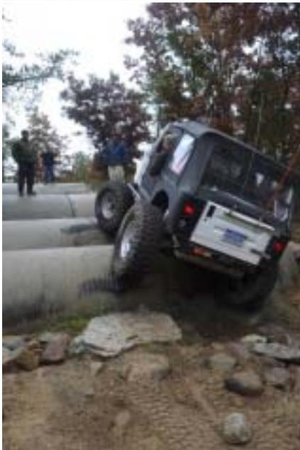
*The rocks approaching the tube course had been pushed out making it just about impossible for even the most built rigs when approaching the run straight on. The new approach is two levels of 2x2x3 concrete blocks that are "stepped", with a small rock scramble below that. Now a rig on 37" tires can approach the obstacle head on and be able to successfully crest the first tube.*
