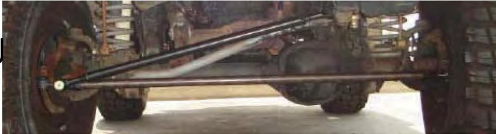
Rugged Ridge's steering linkage assembly "dwarfs" the factory original and give you virtually 1-ton strength with a factory tapered end, so no modifications are necessary! This is a bolt-on solution for preventing bent tie rods and drag links from wheeling with larger tires.
